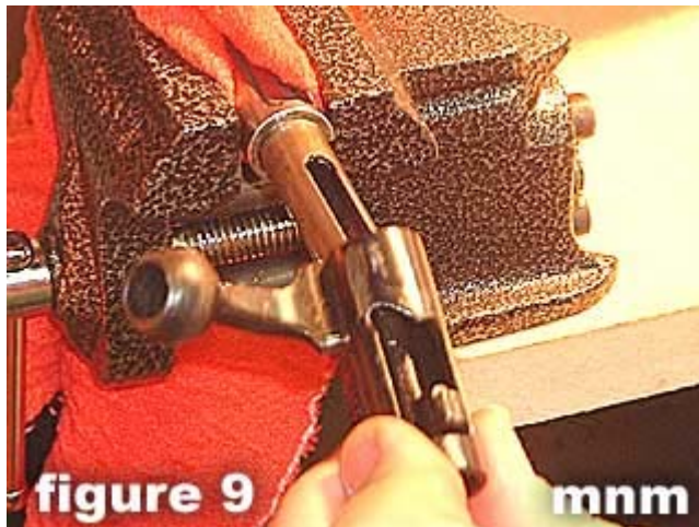
9) Remove the bolt handle and spring follower .
