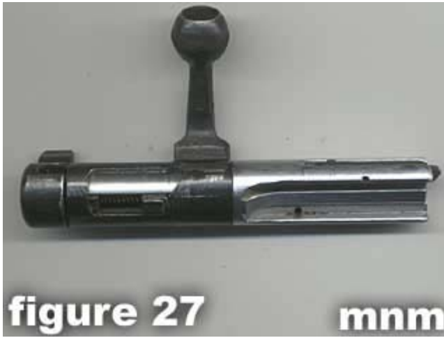
27) Figure 27 shows the reassembled bolt .
