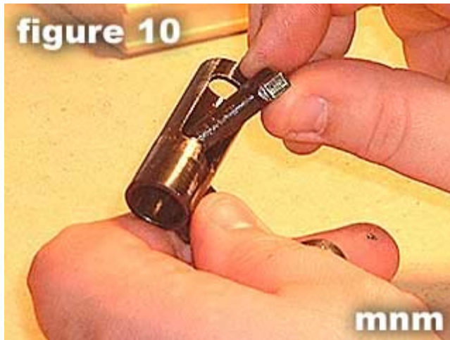
10) Separate the spring follower from the bolt handle (as shown in figure 10 ).
